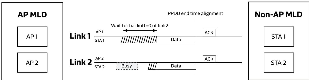
Figure 5. Uplink Transmission to STR AP from NSTR STA
