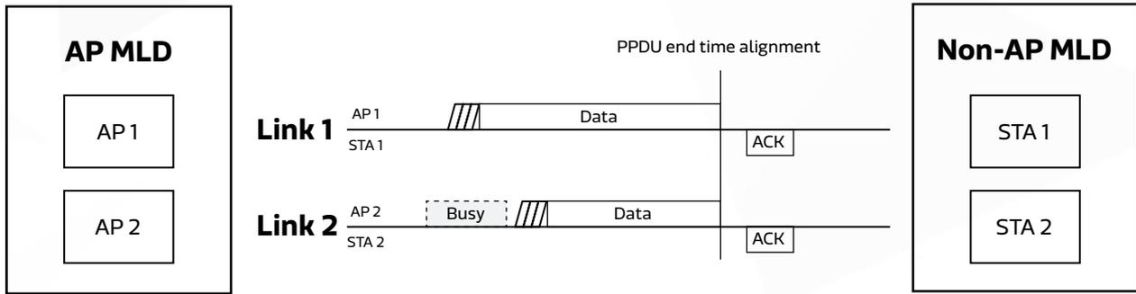
Figure 4. Downlink Transmission from STR AP to NSTR STA
