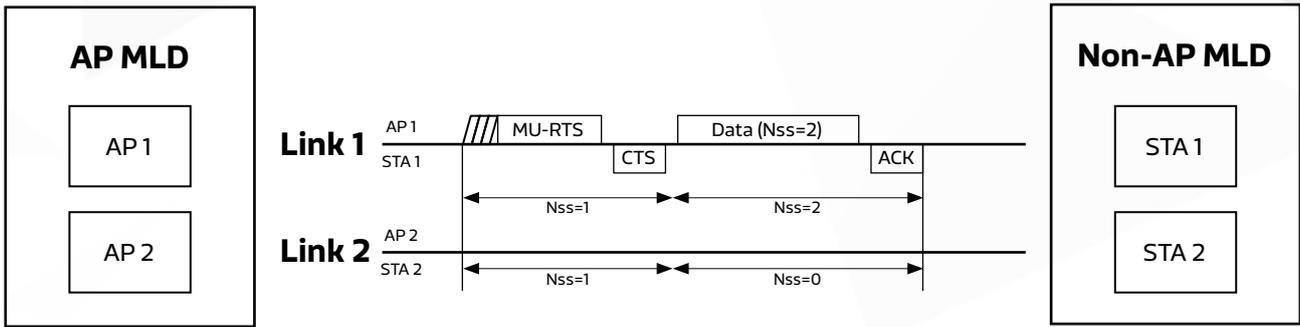
Figure 6. Downlink Transmission from STR AP to EMLSR STA (Max. NSS=2)
