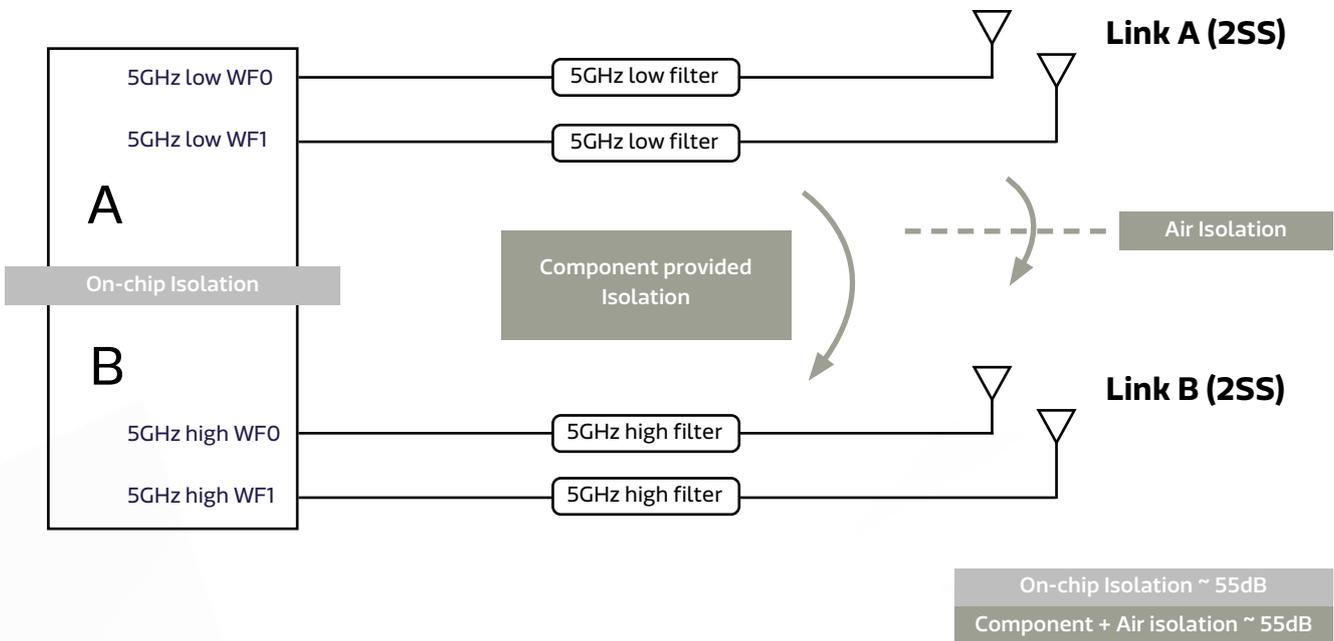
Figure 10. A Quad-Antenna STR STA with 5GHz-High 2NSS + 5GHz-Low 2NSS
