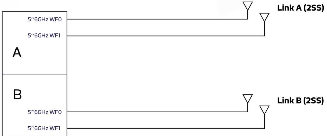
Figure 9. A Quad-Antenna NSTR (or EMLSR) STA with 5/6GHz 2NSS + 5/6GHz 2NSS
