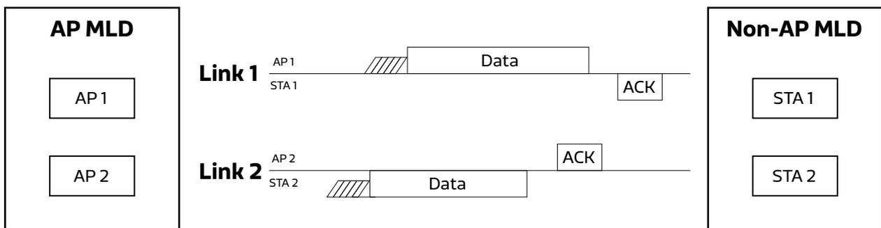
**Figure 1. An Example of MLO Operation with Two Links**
