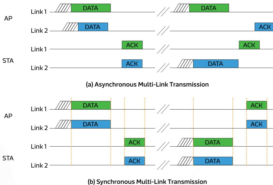
**Figure 2. Multi-Link Transmission: Asynchronous and Synchronous Modes**
