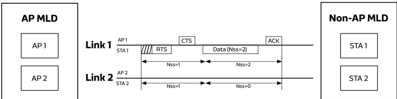
Figure 7. Uplink Transmission from EMLSR STA to STR AP (Max. NSS=2)
