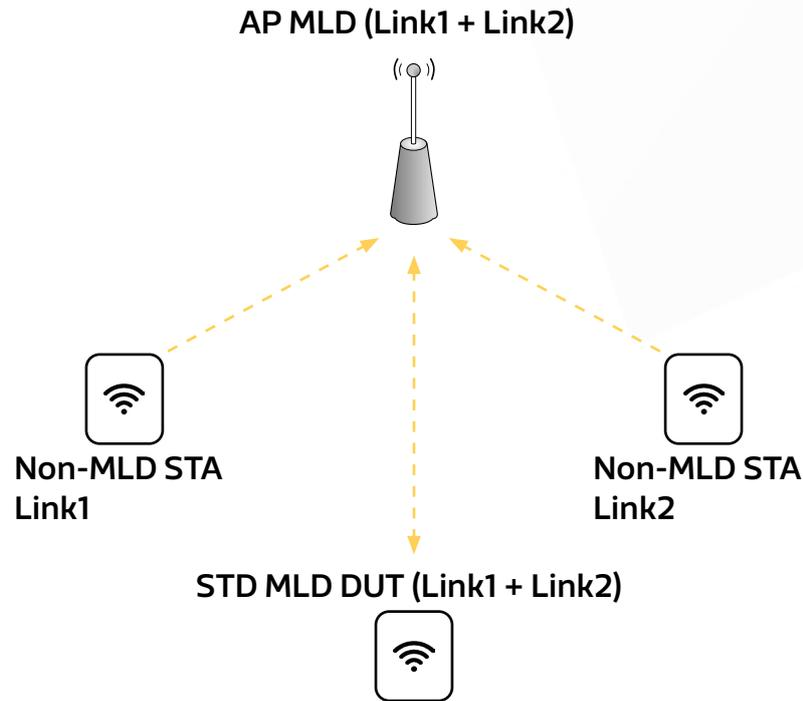
**Figure 8. Network Topology for Simulations**
