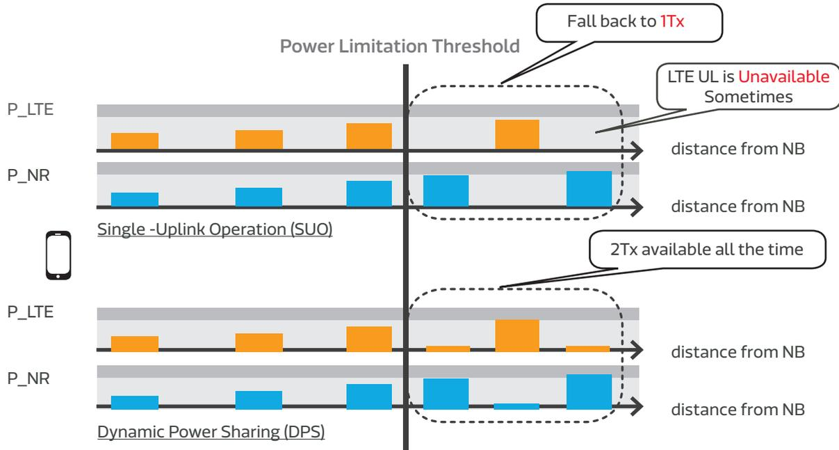
Figure 8 SUO and DPS Operation
