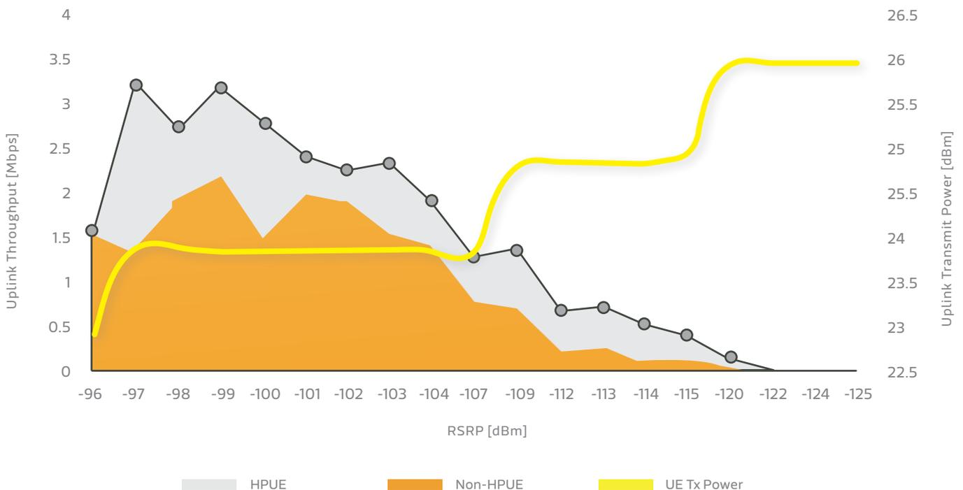
Figure 1- HPUE vs. non-HPUE Uplink Throughput Performance in Mobility
