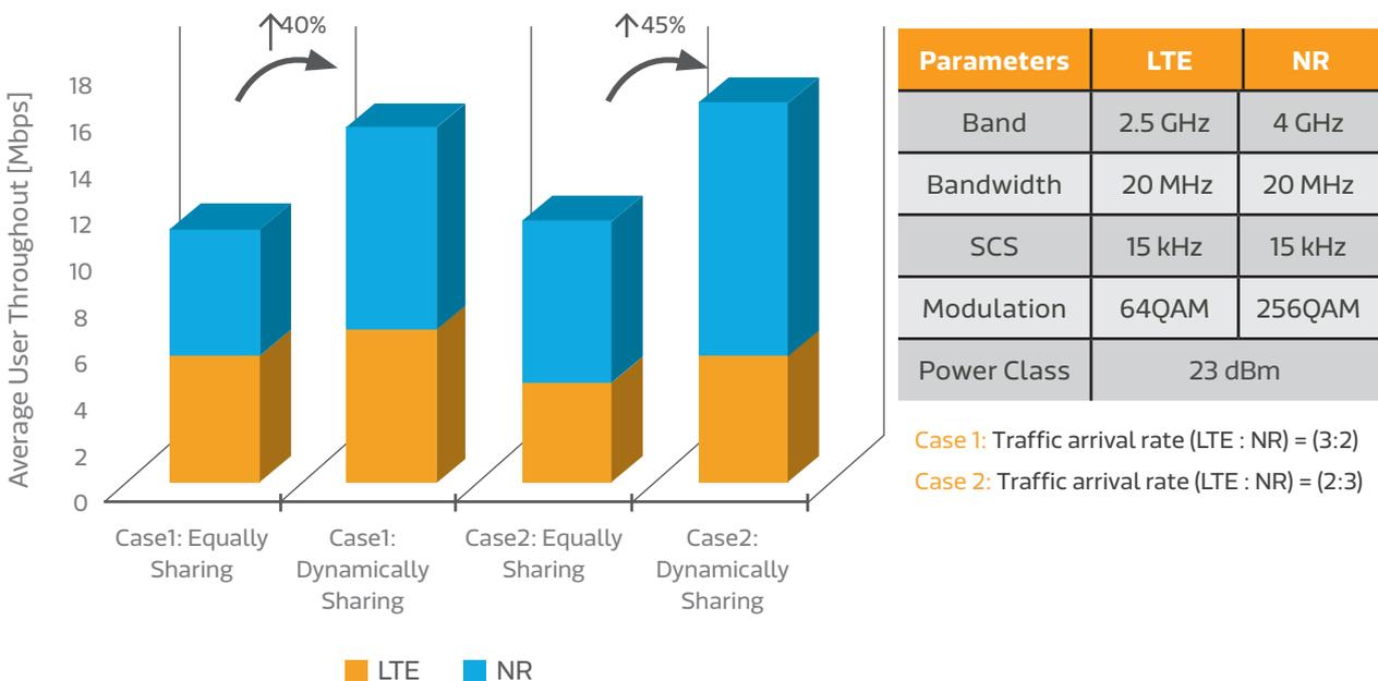
Figure 4 EPS vs. DPS, Average User Throughput Comparison
