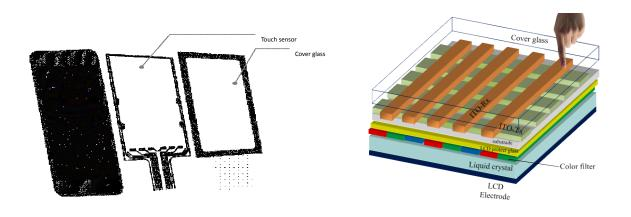
ITO-Tx sends signal out while ITO-Rx receives for touch detection. Finger touching disturbs ITO-Rx receiving, creating the touch event. The graphic below shows the interaction between the TX and RX grids on separate screens during HotKnot mode.
