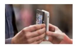
NFC has several limitations. As shown here, NFC sharing requires back-to-back because the display shields NFC signals. Aligning the NFC's antenna's correctly to insure pairing poses difficulties for the users, resulting frequent in pairing failure.
