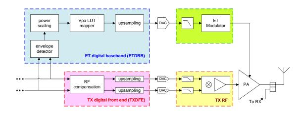
Figure 3. MediaTek's Envelope Tracking System Block Diagram
