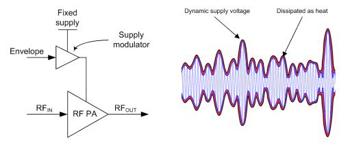
Figure 2. Envelope Tracking Power Amplifier with Dynamic Supply Voltage
