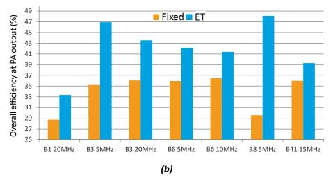
Figure 4: Performance Comparison of Conventional PA and Envelope Tracking PA (a) E-UTRA ACLR and (b) Overall Efficiency
