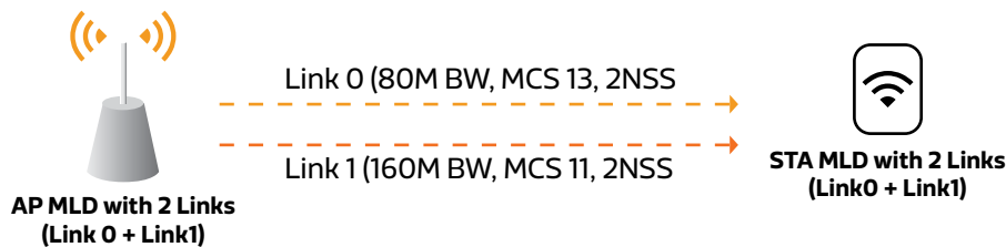
Figure 4. Network Topology of Links with Clean Channels
