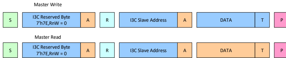
Figure 3-103 I3C SDR Private Write/Read
